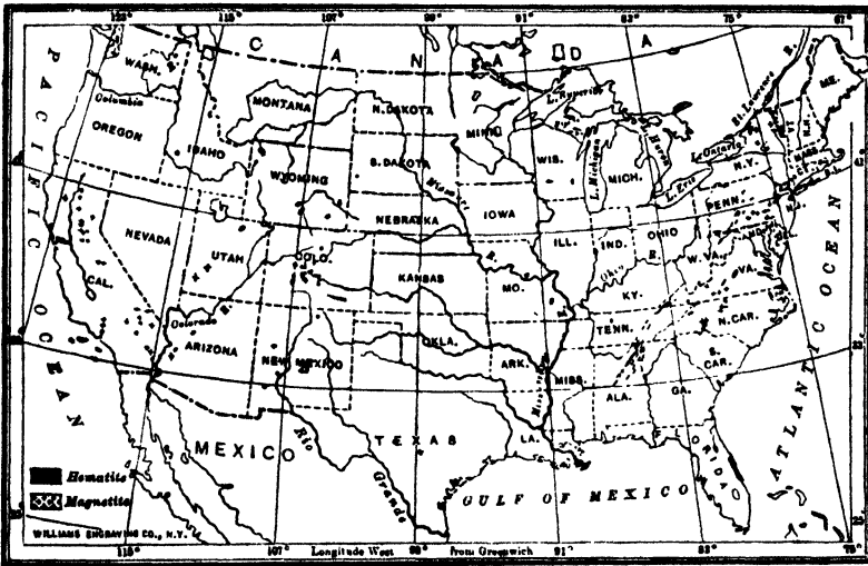
FIG. 127.—Map showing distribution of hematite and magnetite deposits in the United States. (After Harder, U. S. Geol. Surv., Min. Res. , 1907).
